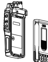
When disassemble batteries, press the release gate, remove the batteries from the radios.
