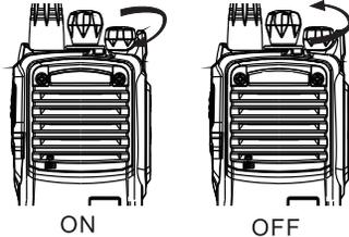
Switch on: rotate the on/off switch clockwise to boot the radios, it will be a boot prompt if the radio works normally and start the boot prompt function, otherwise, there is no boot prompt.
