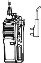
Insert the speaker/microphone plug into SP/MIC jack.
