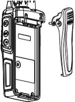
Lock the belt clip onto the up back of the radios, until tighten up.
