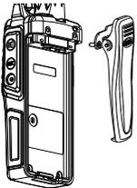
Disassemble these two screws from the belt clip by the screwdriver.
