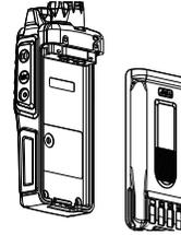
1. Aligned the corresponding notches with the two raised radio end point on the battery pack.
