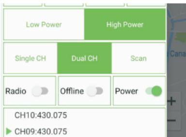
Open the mobile app, click on the [Power] section and turn it to gray to turn off the car radio. The next time you need to turn it on, open the app and the [Power] part will light up and you can use it normally.
