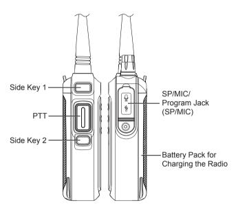
**Remark:** Different functions of Side Key 1, Side Key 2, which are used by the long press or a short press, can be defined by programming software.
